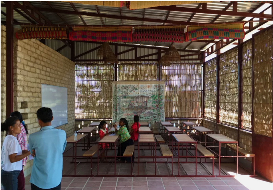
the teaching space can be divided into two classrooms by lowering woven mat screens, or used as one large hall
